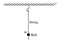
• The bob begins to move to and fro when it is released from the extreme position **II** i.e., it will go up to another extreme position **III** via mean position **I**, and then go up to position **II** again via mean position **I**. It will continue to move in the same way. This back and forth motion of the bob via mean position **I** is called the **periodic or the oscillatory motion of the bob**.
